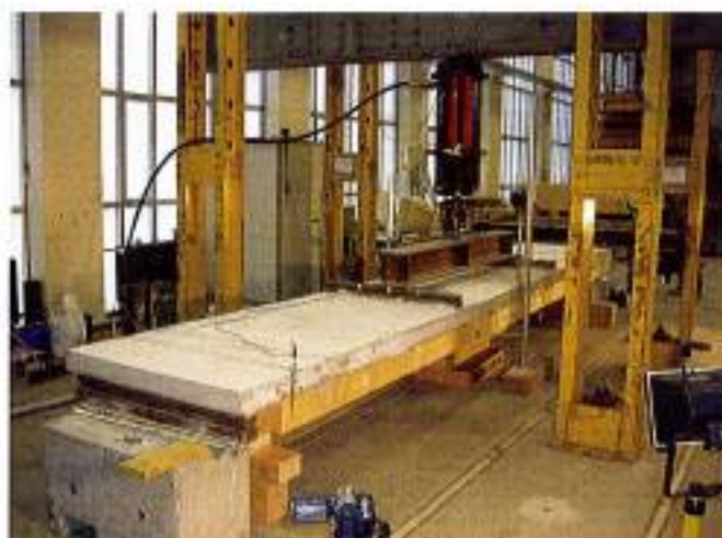
Bild 17. Deckenstreifen in der Prüfmaschine Fig.17. Timber-concrete-composite ceiling during testing
